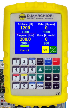
Optional MPSRC Hand held remote control unit: Multi-coloured backlit 3.5" LCD touchscreen and keypad
